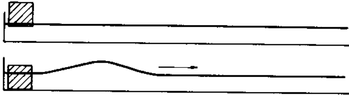
Figure 3: The diagram of Russel's experiment to generate solitary waves
